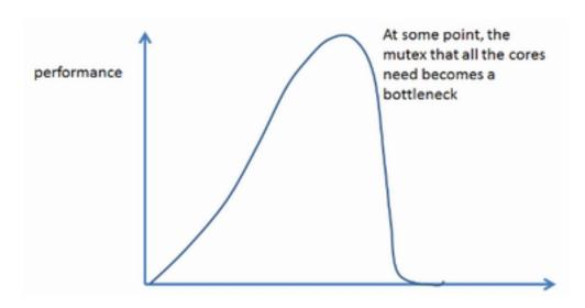
After a certain point, adding cores causes the performance to crash. (lots of time to go from one core to the next because the mutex that all the cores need becomes bottleneck Solution to contention problems: Try to remove the locks (try to work without having to use locks) or minimize the execution time of the code in critical sections.
