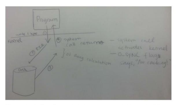
[diagram showing forced interaction between program and disk on each call to write() because of O\_SYNC flag]
