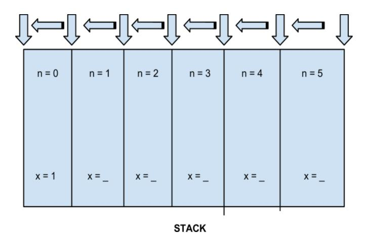
Now we move back up the stack by intervals of sizeof(factorial\_args\_and\_locals) setting x = previous x \* n for each struct.
